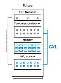
Figure 5 Composable architecture extended to the rack
