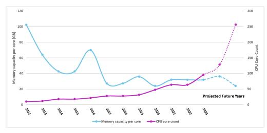
Figure 2 Historical trend lines for typical system memory capacity and CPU core count (Source: Based on capacity and core counts from publicly available AMD and Intel datasheets, and public statements.)
