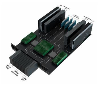
Figure 4 CXL enabled server with CXL memory modules
